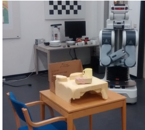
Fig. 1. PR2 during a search process. The target volume on top of the table has several occlusions and a cavity.
