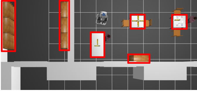
Fig. 4. Top-down view of the simulated environment used in the experiments, consisting of two connected rooms with various target volumes (red boxes: two shelf arrangements, one single shelf, three cluttered tables).
